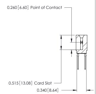
ACAD REFERENCE NO. 746 Series Ultra-Mate Card Edge Connector - Press Fit DRAWN: J.LEE Part Number: 746-046-540-201 CHECKED: **EDAC INC** SCALE: THESE DRAWINGS AND SPECIFICATIONS ARE THE PROPERTY OF EDAC INC.,AND TORONTO, ONTARIO SHALL NOT BE REPRODUCED, OR COPIED DRAWING NUMBER CANADA OR USED AS THE BASIS FOR THE 746-ENG MASTER MANUFACTURE OR SALE OF APPARATUS
