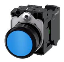
Pushbutton, 22 mm, round, plastic, blue, pushbutton, flat, momentary contact type, with holder 1 NO, spring-type terminal, with laser labeling, lower case
