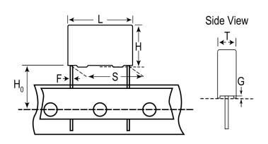
Series F881 Dielectric Metallized Polypropylene Style Radial Features MKP, Pulse RoHS Yes Wire Leads Lead Safety Class Qualifications ENEC, UL, cUL, CQC AEC-Q200 No THB Performance No Component Weight 1.121 g Miscellaneous ClimCat: 40/110/56/C. Shelf Life 104 Weeks
