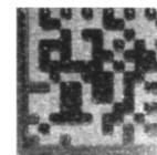
Comparison of direct part mark and Data Matrix after processing
