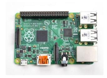
Start by plugging the 2x20 header into a Raspberry Pi, this will keep the header stable while you solder. Make sure the Pi is powered off!
