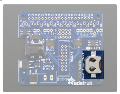
The rgb-matrix.sh script already installed the necessary software to use the realtime clock...but you'll need to set the initial time once. This is explained in the "Sy nc time from Pi to RTC" section of this DS1307 tutorial () (just that one section...you can ignore the rest).
