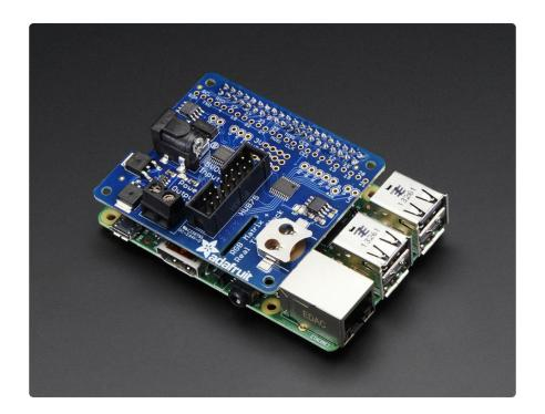
Works with any of our 16x32, 32x32 or 32x64 RGB LED Matrices with HUB75 connections (). The latest "Rev C" HAT also supports 64x64 matrices by soldering a small jumper on the PCB. You can even chain multiple matrices together for a longer display - we've only tested up to 32x128 but it works just fine. The bigger the display the harder it is on the Pi, so keep that in mind if you're using a lower-powered Pi Zero.
