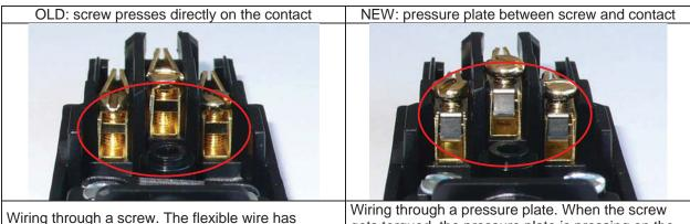
Wiring through a screw. The flexible wire has tendencies to move on one side.
