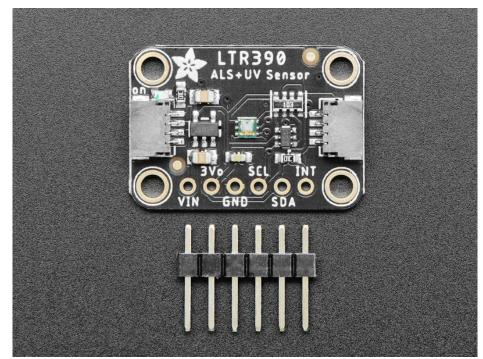
Unlike sensors that estimate UV Index readings from visible and IR light levels such as the Si1145 (http://adafru.it/1777), the LTR390 incorporates two sensors, one for visible and another specifically designed to measure UV light levels. The sensor's CircuitPython library includes routines to derive the UV Index value from raw UV measurements as well as calculating the ambient light Lux level.
