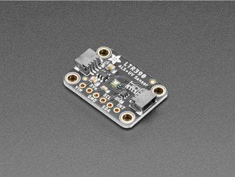
The LTR390 (https://adafru.it/PBv) is one of the few low-cost UV sensors available, and it's a pretty nice one! With both ambient light and UVA sensing with a peak spectral response between 300 and 350nm. You can use it for measuring how much sun you can get before needing to covering up.
