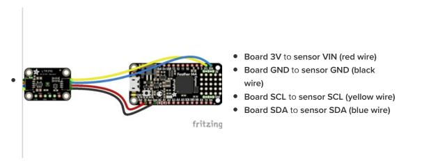
You can also use the standard **0.100" pitch** headers to wire it up on a breadboard:
