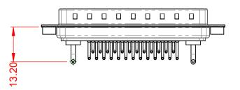
10A (CURRENT) POWER/CO-AX CONTACT RATING: (IF PRESENT) SIGNAL CONTACT CURRENT RATING: 5A PER CONTACT SIGNAL CONTACT RESISTANCE:  $10m\Omega$  MAX. **INSULATOR RESISTANCE:** 5000MΩ min.
