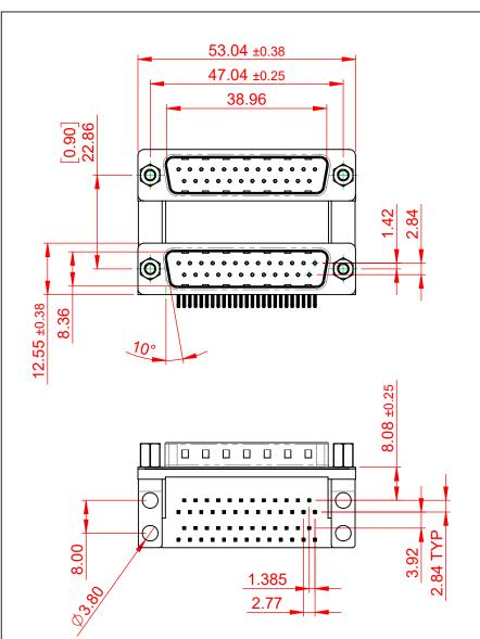
THIS IS A C.A.D. GENERATED DRAWING TOLERANCE UNLESS OTHERWISE SPECIFIED DO NOT MAKE MANUAL REVISIONS TO MASTER. .X ±0.25 .XX ±0.13 .XXX ±0.10
