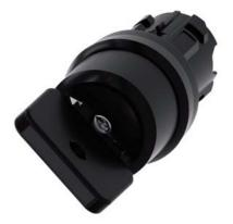
Key-operated switch O.M.R, 22 mm, round, plastic, lock number 73034, black, with 2 keys, 2 switch positions O-I, latching, actuating angle  $90^\circ$ , 10:30h/13:30h, key removal O, with laser labeling, lower case
