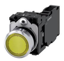
Illuminated pushbutton, 22 mm, round, metal, shiny, yellow, pushbutton, flat, momentary contact type, with holder, 1 NO+1 NC, LED module with integrated LED 24 V AC/DC, screw terminal, with laser labeling, symbol number according to, ISO 7000 or IEC 60417
