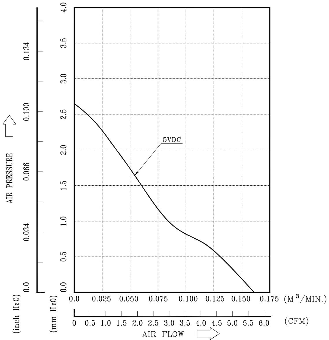
\*TEST CONDITION: INPUT VOLTAGE-----OPERATION VOLTAGE
