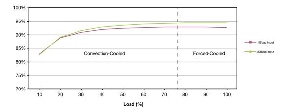
Figure 2 ECP130PS24 24 V at 130 W
