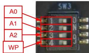
Figure 7. EEPROM Switches in their Defaults Positions. The First Switch (A0) of SW1 is ON, the Second Switch(A1) is ON, the Third switch (A2) is OFF, and the Fourth Switch (WP) is ON
