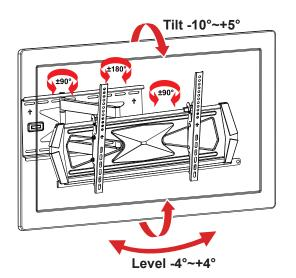
Adjust to the desired position by tilting -10° $\sim$ +5°, swiveling -90° $\sim$ +90°, -180° $\sim$ +180°, -90° $\sim$ +90° at three pivot points,and by leveling -4° $\sim$ +4°.
