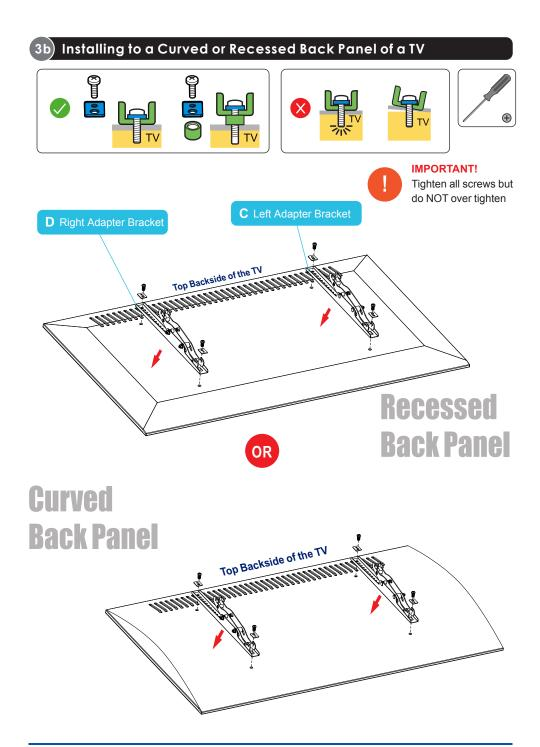
Choose the appropriate screws, washers, and spacers (if necessary) according to the type of your TV and attach adapter brackets (C and D) to the back of the TV using a Phillips screwdriver.
