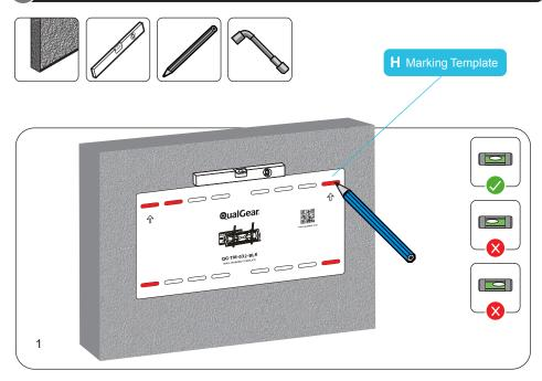
Hold the marking template (H) provided against the wall where you want to install the TV, mark five holes for drilling.
