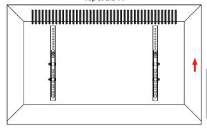
According to the direction indicator arrows on the adapter brackets, make sure the adapter brackets are installed in the correct direction.
