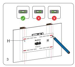
Using the marking template (H) provided, mark four holes for drilling on the centerline of the stud.
