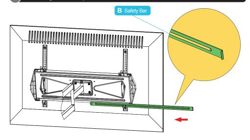
Insert the safety bar onto the rail (at the bottom of the wall plate) to secure.
