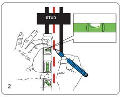
Using a level, mark the centerline of the stud.
