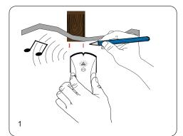
Using an edge-to-edge stud finder, find the edges of the stud.
