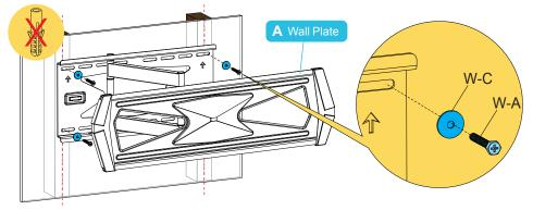
5 Mount the wall mount (A) and tighten it with the provided lag bolts (W-A) and D6 washers (W-C) using a socket wrench.
