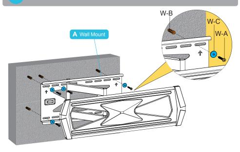
3 Place concrete anchors (W-B) in each hole. Tap each anchor flush with the wall using a hammer. Using a socket wrench, mount the wall mount (A) and fasten them with the provided lag bolts (W-A) and D6 washers (W-C).
