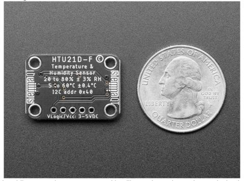
This I2C digital humidity sensor is an accurate and intelligent alternative to the much simpler Humidity and Temperature Sensor - SHT15 Breakout (http://adafru.it/1638) It has a typical accuracy of  $\pm 2\%$  with an operating range that's optimized from 5% to 95% RH. Operation outside this range is still possible - just the accuracy might drop a bit. The temperature output has an accuracy of  $\pm 1^{\circ}$ C from -30~90°C. If you're
