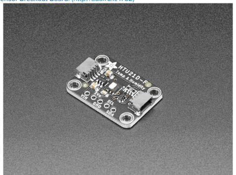
Such a lovely chip - so we spun up a breakout board that includes the Filtered version (the white bit of plastic which is a PTFE filter to keep the sensor clean), a 3.3V regulator and I2C level shifting circuitry. This lets you use it safely with any kind of microcontroller with 3.3V-5V power or logic.
