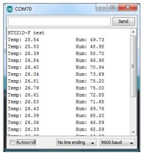
You can try breathing on the sensor to increase the humidity. The sensor reacts very fast!
