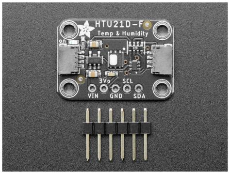
To get you going fast, we spun up a custom made PCB in the **STEMMA QT** form factor (https://adafru.it/LBQ), making them easy to interface with. The STEMMA QT connectors (https://adafru.it/JqB) on either side are compatible with the SparkFun Qwiic (https://adafru.it/Fpw) I2C connectors. This allows you to make solderless connections between
