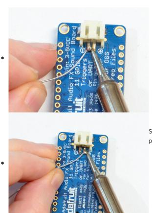
Solder all four pads - two mechanicals on the side, and two power coming out the end.
