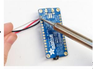
Solder both wires securely. You **cannot** just twist the wires into place!
