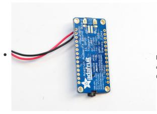
For most battery packs the red wire is the positive wire, connect that to Vin. The black wire is ground, connect that to GND.
