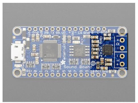
All the way to the right is the Class D stereo amplifier. This is for connecting to a pair of speaker! The outputs are bridge-tied-load (BTL) so do not connect R+ to L+ and R- to L- to get more power, it could damage the chip. If you only need one speaker, simply connect the channel you want.
