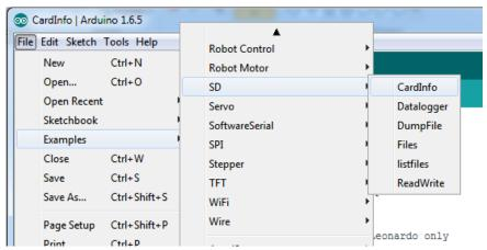
Luckily many of the default examples already have **chipSelect = 4** so you can just upload immediately. For other sketches, do check to make sure that CS is set to 4! The SD card uses hardware SPI for the remaining pins.
