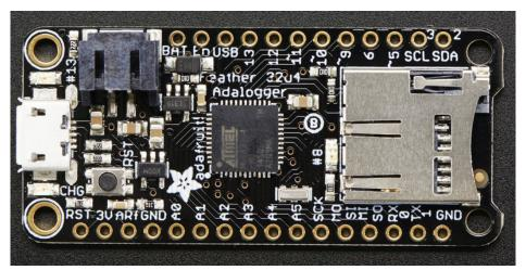
At the Feather 32u4's heart is at ATmega32u4 clocked at 8 MHz and at 3.3V logic, a chip setup we've had tons of experience with as it's the same as the Flora (https://adafru.it/dVI). This chip has 32K of flash and 2K of RAM, with built in USB so not only does it have a USB-to-Serial program & debug capability built in with no need for an FTDI-like chip, it can also act like a mouse, keyboard, USB MIDI device, etc.
