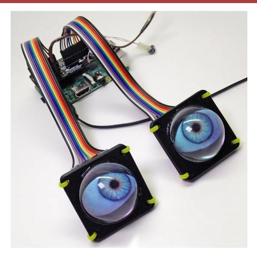
The *Snake Eyes Bonnet* is a **Raspberry Pi accessory** for driving **two** 128x128 pixel OLED *or* TFT LCD displays, and also provides four **analog inputs** for sensors.
