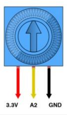
For manual control of pupil dilation (instead of responding to light) a 10K potentiometer can be used. The center leg connects to analog pin A2 (same input as the photocell, just substituting a different analog control).
