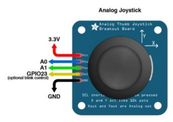
**XOUT** and **YOUT** from a joystick can connect to analog pins **A0** and **A1**.
