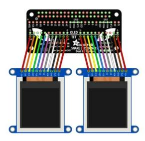
There's a common trope in science fiction stories: that there is no "up" or "down" in space. Wiring these displays is a little like that...it doesn't matter if the wires or headers come out the *front* or *back* of the display breakout board, use *straight* or *right-angle* pins...as long as those wires get from the display to the bonnet in the **same positions and order**, everything's good.
