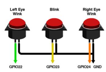
For all buttons, connect one leg of each to **GND**, and the opposite leg to a digital pin:
