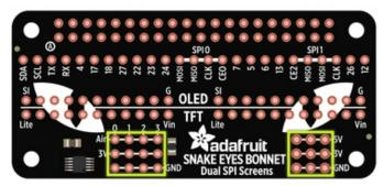
At the bottom-right of the bonnet are a few extra connection points for **5 Volts**, **3.3 Volts** and **ground**, if you have a circuit that needs them. These are OK for **small loads** like ICs or a few LEDs, but *not* for big things like servos, which will need their own power source.
