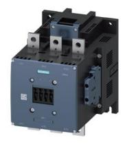
Contactor, AC-1, 690 A/690 V/40 °C, S12, 3-pole, 500-550 V AC/DC, with varistor, 2 NO+2 NC, Connection rail/ screw terminal
