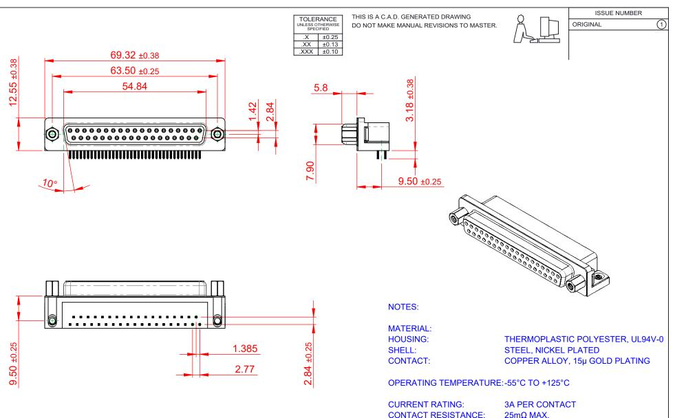
CONTACT RESISTANCE: **INSULATOR RESISTANCE:** 5000MΩ min. DIELECTRIC WITHSTANDING VOLTAGE: 1000V AC rms
