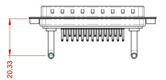
POWER/CO-AX CONTACT RATING: (IF PRESENT) SIGNAL CONTACT CURRENT RATING: 5A PER CONTACT SIGNAL CONTACT RESISTANCE:  $10m\Omega$  MAX. **INSULATOR RESISTANCE:** 5000MΩ min. DIELECTRIC
