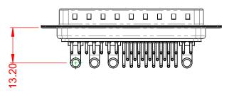
40A (CURRENT) POWER/CO-AX CONTACT RATING: (IF PRESENT) SIGNAL CONTACT CURRENT RATING: 5A PER CONTACT SIGNAL CONTACT RESISTANCE:  $10m\Omega$  MAX. INSULATOR RESISTANCE: 5000MΩ min.
