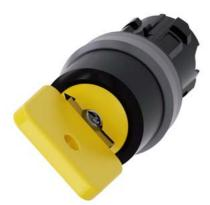
Key-operated switch O.M.R, 22 mm, round, plastic with metal front ring, lock number 73033, yellow, with 2 keys, 2 switch positions O<I, momentary contact type, Actuating angle 45°, 10:30h/12h, key removal O, with laser labeling, lower case
