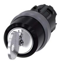
RONIS key-operated switch, 22 mm, round, plastic with metal front ring, lock number SB30, with 2 keys, 3 switch positions I-O-II, latching, actuating angle 2x45°, 10:30h/12h/13:30h, Key removal I+O+II, possible special locks: SB31, 421, 455, with laser labeling, lower case
