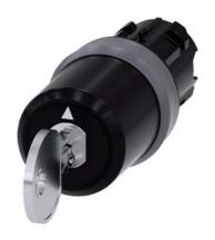
key-operated switch Siemens, 22 mm, round, plastic with metal front ring, lock number SSG10, with 2 keys, 3 switch positions I-O<II, left latching, momentary contact type on the right, actuating angle 2x45°, 10:30h/12h/13:30h, key removal I, with laser labeling, inscription or symbol customer-specific selection with SIRIUS ACT configurator (CIN)
