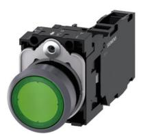
Illuminated pushbutton, 22 mm, round, plastic with metal front ring, green, pushbutton, flat, momentary contact type, with holder, 1 NO+1 NC, LED module with integrated LED 110 V AC, screw terminal, with laser labeling, lower case
