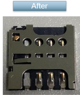
1.27µm min-2.54µm max. matte tin on solder tail over 1.27µm min. nickel underplate over all
