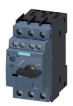
Special type Circuit breaker size S0 for motor protection, CLASS 10 A-release 27...32 A N-release 400 A screw terminal Standard switching capacity with transverse auxiliary switches 1 NO+1 NC Ambient temperature -50 °C 500 switching cycles
