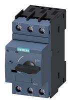
Circuit breaker size S0 for starter combination Rated current 2.5 A N-release 33 A screw terminal Standard switching capacity
