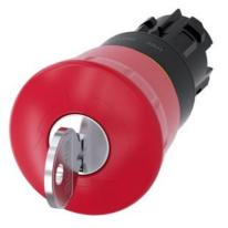
EMERGENCY STOP mushroom pushbutton, 22 mm, round, plastic, red, 40 mm, with RONIS lock, lock number 455, positive latching, acc. to EN ISO 13850, key-operated release Z=50-unit packaging
