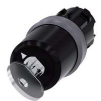
key-operated switch Siemens, 22 mm, round, plastic with metal front ring, lock no. LSG1, with 2 keys, 2 switch positions O<I, momentary contact type, actuating angle 45°, 10:30h/12h, key removal O, with laser labeling, upper case and lower case, always upper case at the beginning of the word
