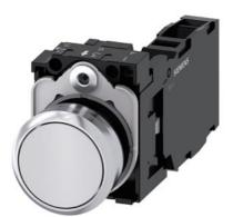
Pushbutton, 22 mm, round, metal, shiny, white, pushbutton, flat, momentary contact type, with holder, 1 NO+1 NC, screw terminal, with laser labeling, upper case and lower case, always upper case at the beginning of the word
