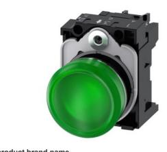
Indicator lights, 22 mm, round, metal, shiny, green, lens, smooth, with holder, LED module with integrated LED 24 V AC/DC, screw terminal, with laser labeling, upper case and lower case, always upper case at the beginning of the word
