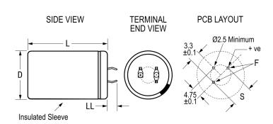
General Information Series ALC70 Dielectric Aluminum Electrolytic Description Snap-In, Aluminum Electrolytic RoHS Lead 3 Pin Short AEC-Q200 No Halogen Free Yes Component Weight 65 g Notes Dimensions D And L Include Sleeving. Shelf Life 156 Weeks
