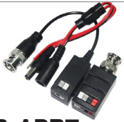
HDB-APRT 5MP Active / Passive Video Balun, CAT5 or Higher CVI 720P 450m (1478ft), 1080P 360m (1181ft) TVI 720/1080P 320m (1049ft) AHD 720P 500m (1640ft), 1080P 360m (1181ft) CVBS 600m (1968ft)
