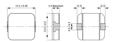
**General Information** Series MPX Style SMD Chip Size 1235(5350) Description Surface Mount Inductor Features Power Inductors **RoHS** Yes Core Composite Miscellaneous 40 (K) Temperature Rise Max.
