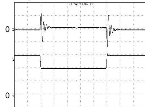
Figure 9: Output voltage response to step-change in load current (75%-50%-75% of I_o , max; di/dt = 1.0A/\mu s ). Load cap: 220 \mu F tantalum capacitor and 1 \mu F ceramic capacitor. Top Trace: V_{out} (100mV/div, 200 \mu s /div), Bottom Trace: I_{out} (10A/div). Scope measurement should be made using a BNC cable (length shorter than 20 inches). Position the load between 51 mm to 76 mm (2 inches to 3 inches) from the module
