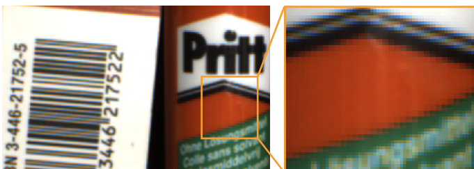
With standard 2x2 debayering, artefacts such as saw-tooth distortion or zip effects compromise the image quality considerably.
