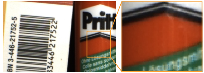
PGI 5x5 debayering clearly improves the edges in the image.
