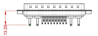
10A (CURRENT) POWER/CO-AX CONTACT RATING: (IF PRESENT) SIGNAL CONTACT CURRENT RATING: 5A PER CONTACT SIGNAL CONTACT RESISTANCE:  $10m\Omega$  MAX. 5000MΩ min. **INSULATOR RESISTANCE:**
