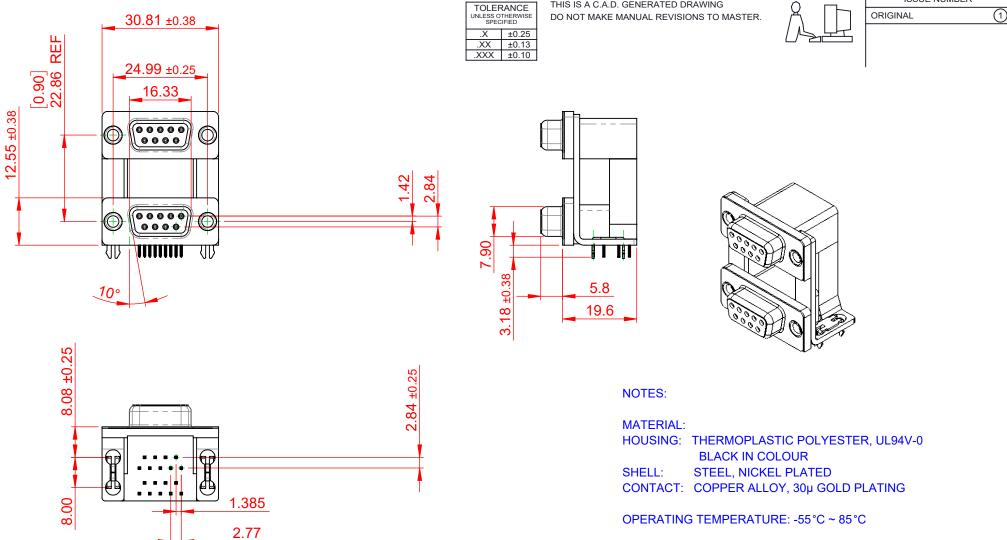
**CURRENT RATING: 3A PER CONTACT** CONTACT RESISTANCE: 25mΩ MAX. INSULATOR RESISTANCE: 5000MΩ min. DIELECTRIC WITHSTANDING VOLTAGE: 1000V AC rms
