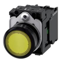
Illuminated pushbutton, 22 mm, round, plastic, yellow, pushbutton, flat, momentary contact type, with holder, 1NO, LED module with integrated LED 110 V AC, screw terminal, with laser labeling, symbol number according to, ISO 7000 or IEC 60417
