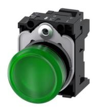
Indicator lights, 22 mm, round, plastic, green, lens, smooth, with holder, LED module, with integrated LED 110 V AC, spring-type terminal, Z=20-unit packaging
