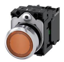
Illuminated pushbutton, 22 mm, round, metal, shiny, amber, pushbutton, flat, momentary contact type, with holder, 1NO, LED module with integrated LED 110 V AC, screw terminal, with laser labeling, symbol number according to, ISO 7000 or IEC 60417
