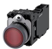
Illuminated pushbutton, 22 mm, round, plastic with metal front ring, red, pushbutton, flat, momentary contact type, with holder, 1 NO+1 NC, LED module with integrated LED 110 V AC, screw terminal, with laser labeling, lower case
