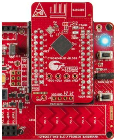
Figure 4-22. RGB LED Control with PSoC 4 BLE Module
