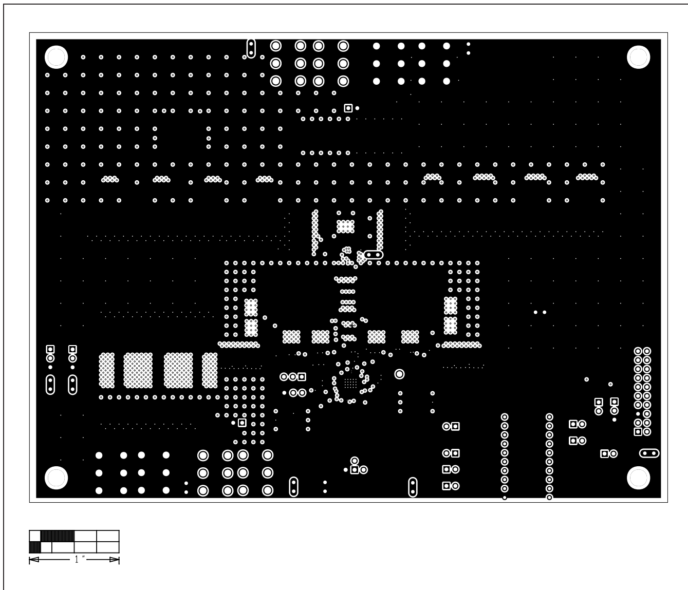
MAX25203 EV Kit PCB Layout—LAYER-2
