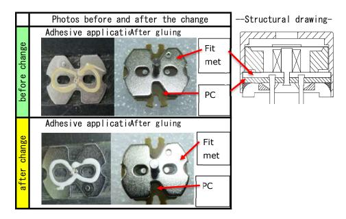
1-2: Fixed strength between metal fittings and PC board The adhesive after the change has a higher fixed strength than the adhesive before the change. The measurement results are shown below.
