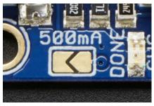
Melt some solder onto the jumper to close it and set the new charge rate
