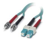
Assembled FO cable, zip cord cable, multimode fiberglass 50/125  $\mu$ m, OM3, plug: SC duplex/B-FOC (ST), degree of protection: IP20, for installation in cable ducts or control cabinets, length: 2 m
